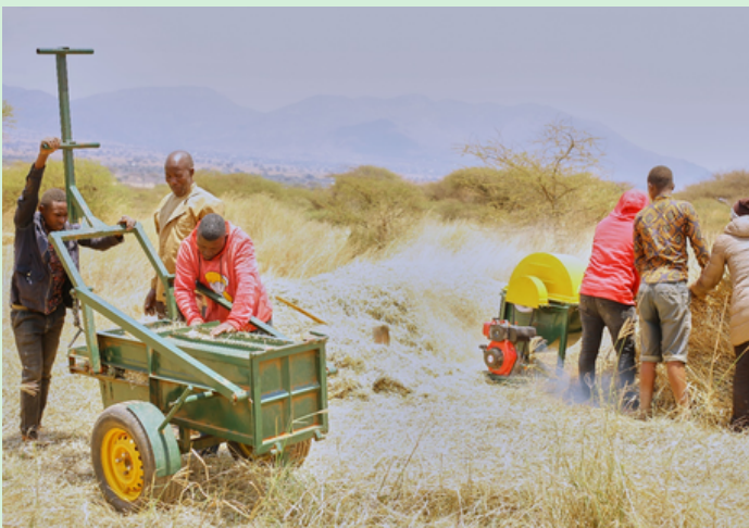
The manual hay baler and grass shredder we provided are being used by villagers in Pembamoto to produce hay bales.
