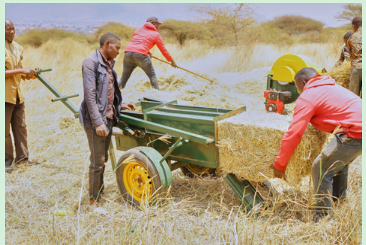
The manual hay baler and grass shredder we provided are being used by villagers in Pembamoto to produce hay bales.
